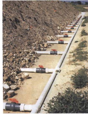
Forced aeration static pile composting of pentachlorophenol contaminated soil at Flinders Bioremediation's dedicated facility at Maslin Beach, SA.
