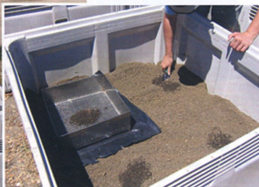
Co-cultures of fungus and bacteria showed promise in trials on 150kg batches of soil contaminated with creosote.
