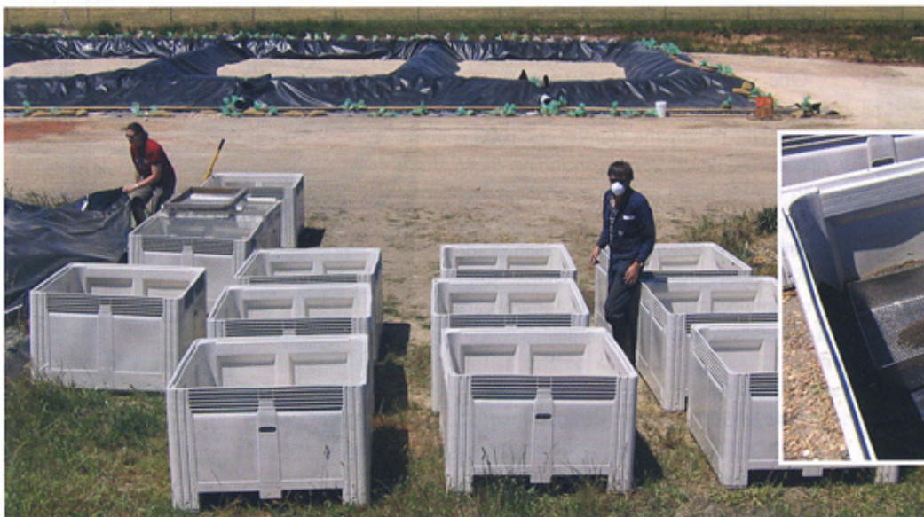
Co-cultures of fungus and bacteria showed promise in trials on 150kg batches of soil contaminated with creosote.
