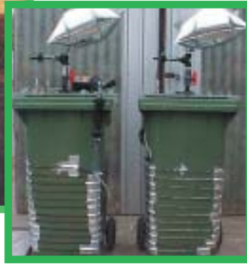
Lab scale anaerobic digestion equipment
